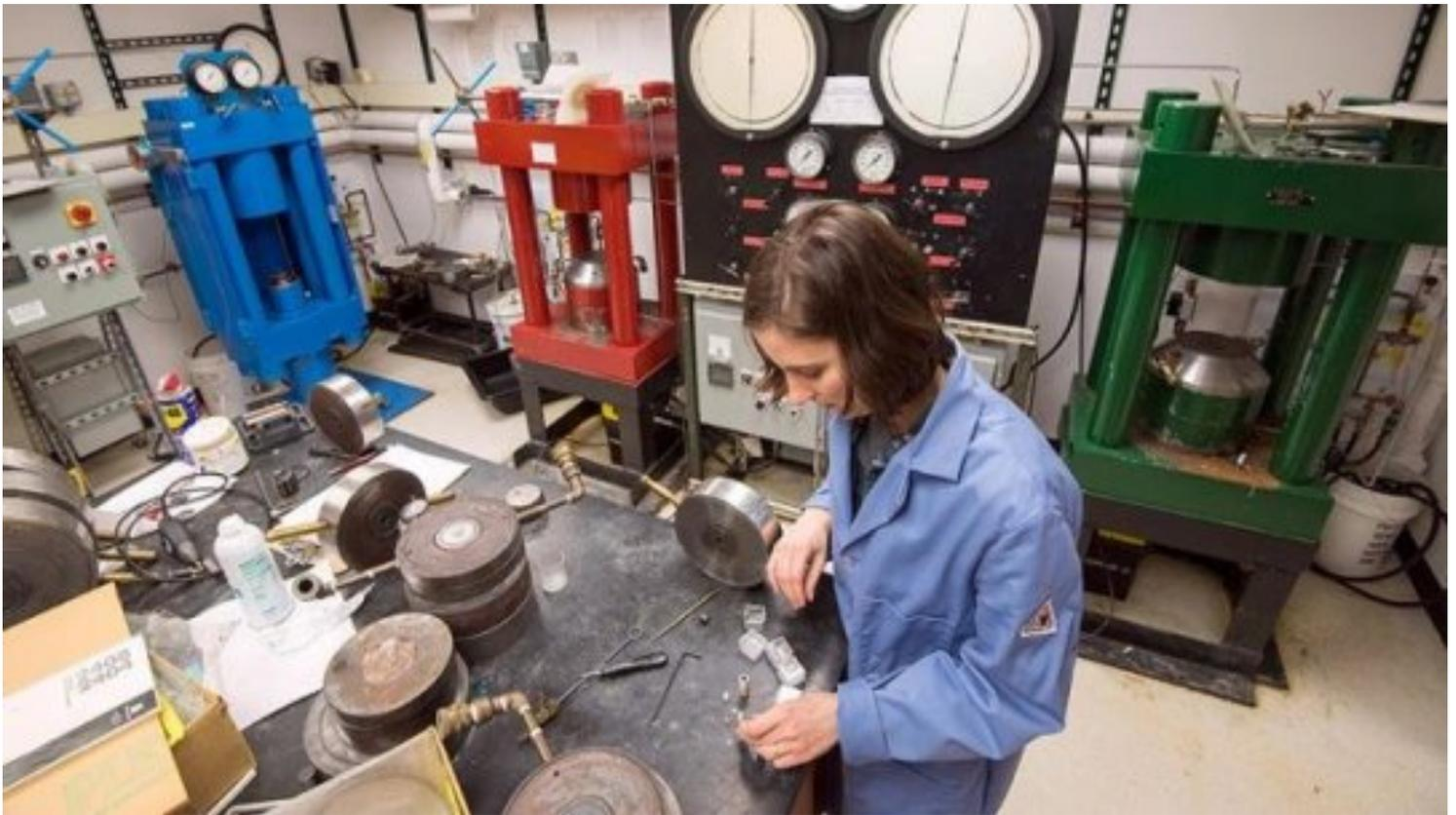
In her laboratory experiments, Sarafian used a piston-cylinder apparatus--the red machine behind her--to simulate the high pressures and temperature of the Earth's mantle. The heavy stainless steel plates visible on the table are stacked on the apparatus, with the tiny synthetic mantle sample inside a 'pressure vessel' underneath them. Once the machine is turned on, pistons apply massive pressure from above and below the sample, which is simultaneously heated with electrical current.
